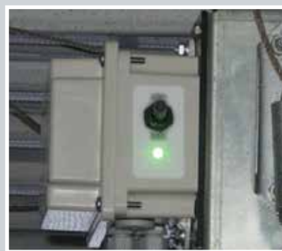
Bi-Color LED allows quick verification of operating status
