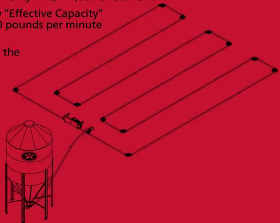
*AP's Flex-Flo™ flexible auger feed delivery system delivers a continuously metered flow of feed from the bin to the Chain Disk system.*
